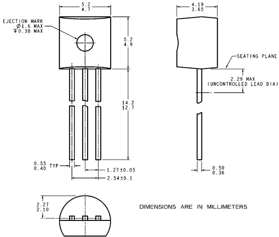
DIMENSIONS ARE IN MILLIMETERS
